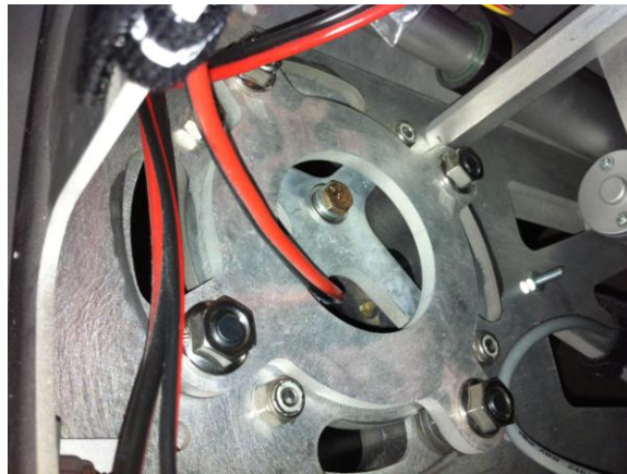
New shoulder lever plate installed, with wired to foot drive passing through the middle. That's what the holes are for ☺
