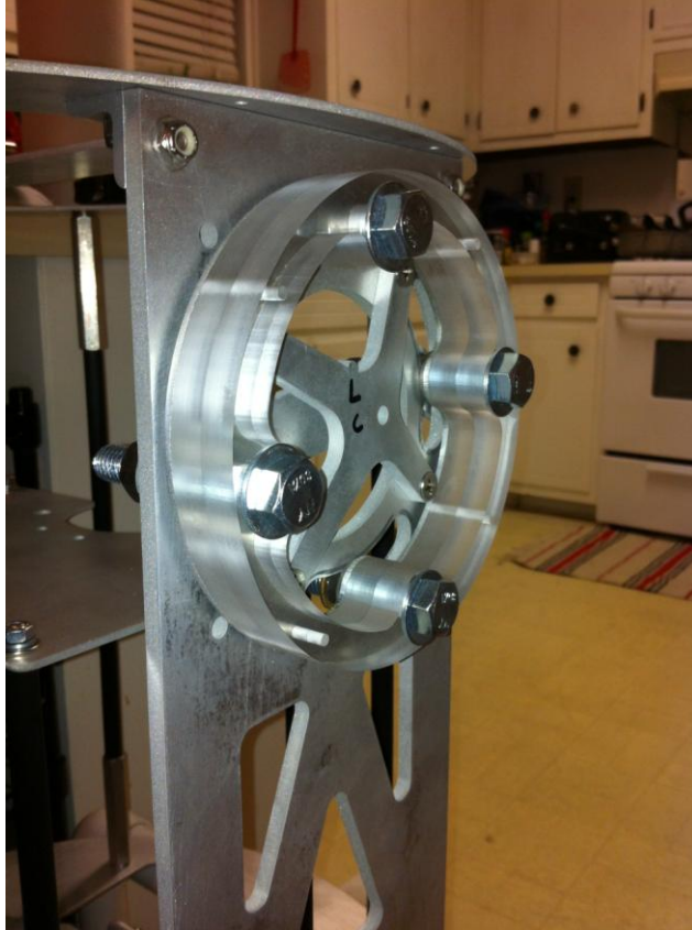
The "spider" inside the leg to body hub, which provides the mounting point to the shoulder for the leg rods.
