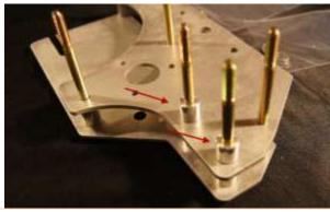
9 Place the completed (and hopefully tightened) caster mount onto these two bolts.
