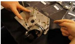
1: You assembly should look like this now. All five of the Part N bolts should have a spacer on them and the caster should be installed with spacer both below and on top.
