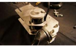
8 This is how the motor should look all seated down with the chain around the sprocket.
