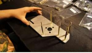
5 Now insert Part P − 10/24" screw and insert it into the upper left hole.
