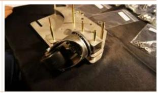
10 Place Part J - 3/8'' spacers on the bolts Part N which go through the caster mount. There are only two bolts.
