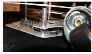
6 Carefully insert the motor into the hole. There is a definite cutout that the wiring will fit through.
