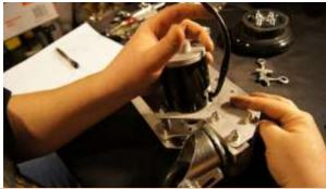
7 The motor should seat down nicely and the wire should have a small amount of play.
