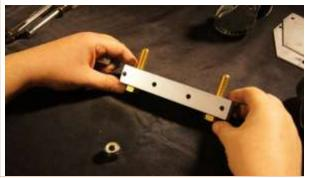
**3** Place the caster on using Part D as the caster shaft. Attach **loosely** with Part E – nylon nut.
