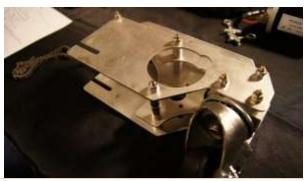
5 With the drive assembly flat on a surface. Carefully lay the chain down ensuring that it is going around the sprocket hole.
