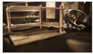
9 Holding the entire assembly, turn it over and carefully move the motor until you line up the mounting holes. There are three. This step is a little awkward as your trying to not lose the chain nor mess up the motor.
