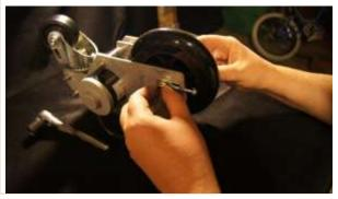
2. Once the axle is in place, go back and tighten up the rest of the motor mount.
