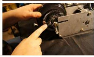
16 The order should be bolt, washer, tensioner, plate, bushing, wheel at this point.
