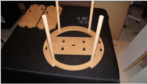
The dowel rods should fit very snugly into the receiving holes.
