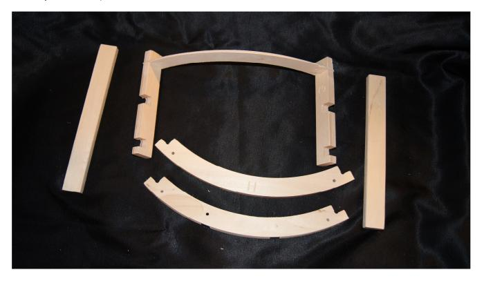
Insert Middle Arm Carrier (H) into the middle notches of the Arm Carrier Sides (G).
