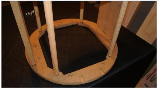
The side plates should fit in first then the dowels. Once you have everything aligned and the dowels slightly inset into the receiver holes, flip the entire assembly over and tap everything into place using the rubber mallet.
