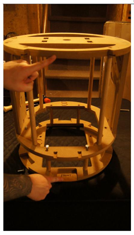
The LDP cutout, the arm carrier notches, and the slot you marked as front should all be aligned.
