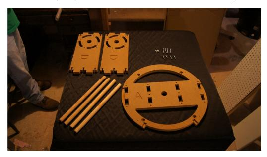
If desired, lightly sand these pieces to remove any sharp edges left over from the CNC machining process.
