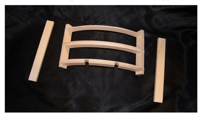
Now insert the Lower Arm Carrier Extensions into the two notches of Lower Arm Carrier (J). You want to pay particular attention and make sure that the fronts of the extensions do not extend past the curvature of the lower arm carrier. You need to do this so your skins will sit flush with the frame.
