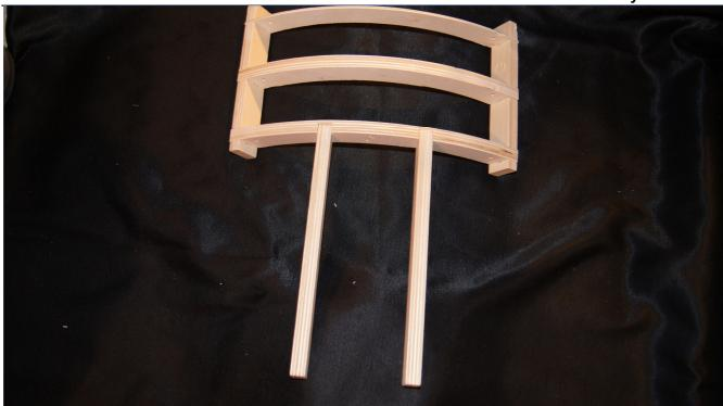
Once you're comfortable with how everything fits together. Carefully take this apart and apply suitable wood glue to each piece and reassemble. The lower arm carrier also has pilot holes drilled if you want to use a small wood screw as well. (I recommend it).
