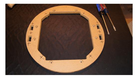
Now get the Top Ring (A) assembly and the Middle Ring (B) and align them as show. The cutout on the Top Ring assembly should face you and the letter 'B' should be to the top.
