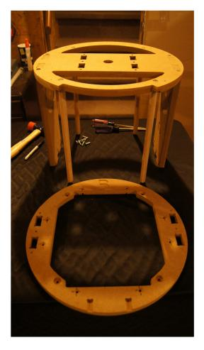
Carefully align the side plates and long dowels into the receiving holes. Take your time on this step.
