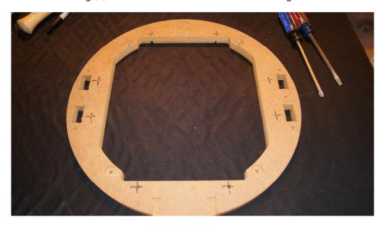
Turn the Middle Ring (B) over and mark and countersink the appropriate holes as shown. The Letter 'B' should be facedown and at the top:
