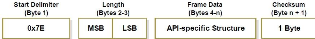
Figure 3-01. UART Data Frame Structure:
