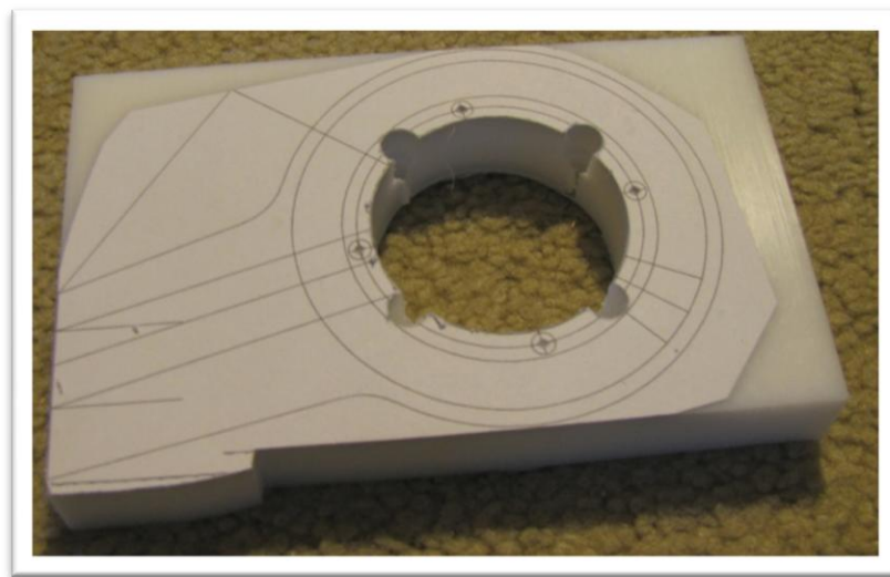
Figure 21: Shoulder lever partially cut and milled
