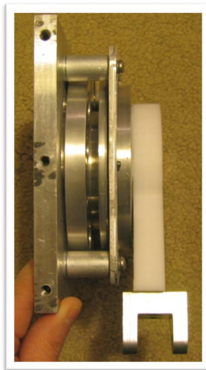
Figure 25: Completed shoulder rotation assembly top view
