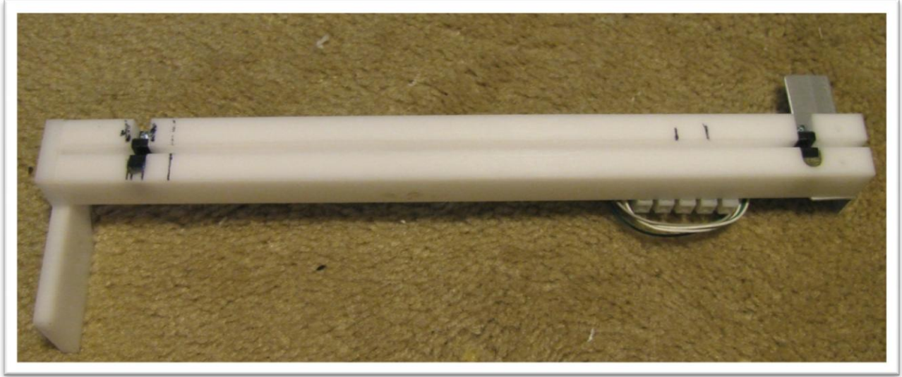
Figure 38: Acetal plastic guide bar for opto-interrupter switches (only 2 switches yet installed)
