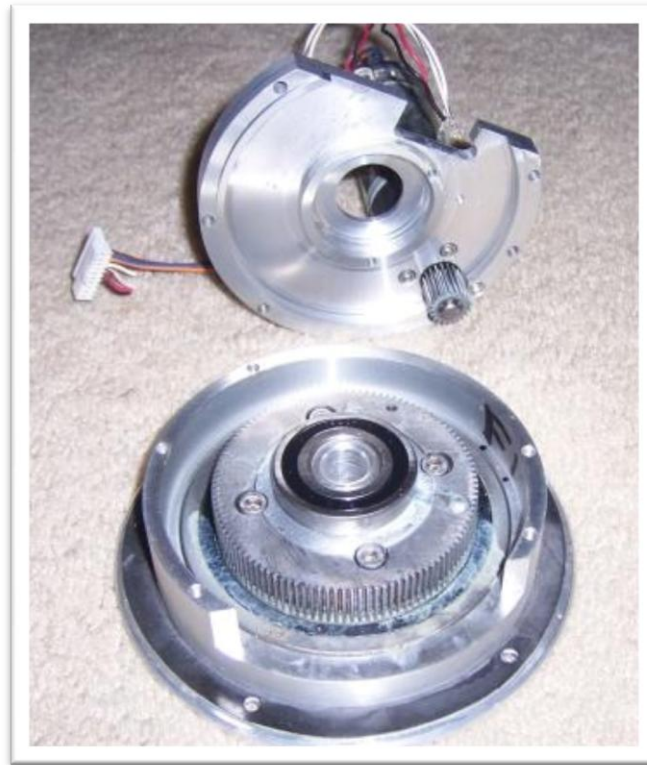
Figure 19: Fine toothed satellite motor gears
