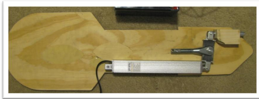
Figure 29: Prototype ankle pin mechanism
