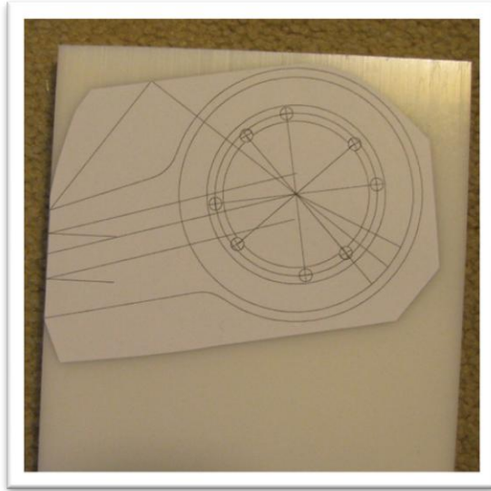
Figure 20: Shoulder lever template and tapped end with clevis mounted
