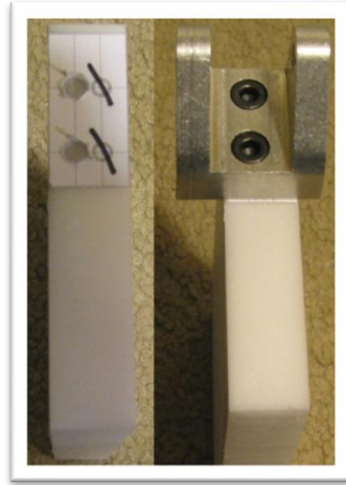
Figure 20: Shoulder lever template and tapped end with clevis mounted
