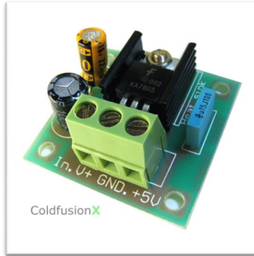
Figure 27: 5V voltage regulators
