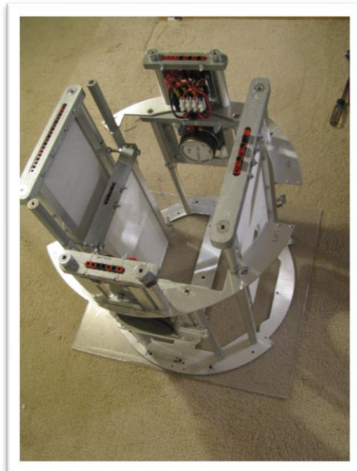
Figure 17: JAG 4 frame with electronic panels mounts – Photo by: Blake Mann
