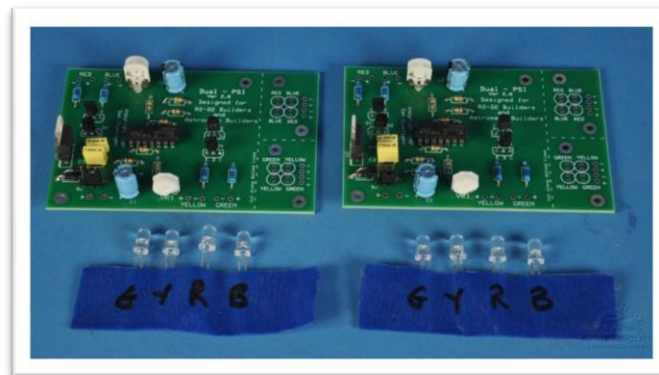
Figure 13: R2 Builders dual PSI circuit boards – Dan S.
