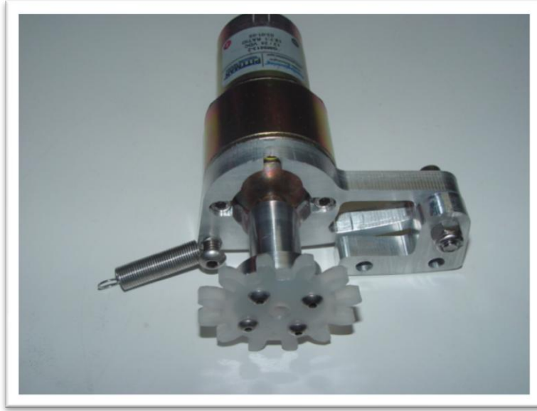
Figure 31: Aluminum dome drive bracket & spring - Photo by: Atomic Pickle
