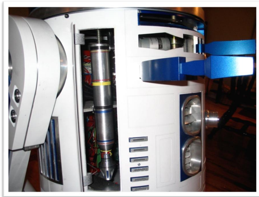
Figure 33: CPU arm mounted behind the front vertical panel - Photo by: Cory Pacione
