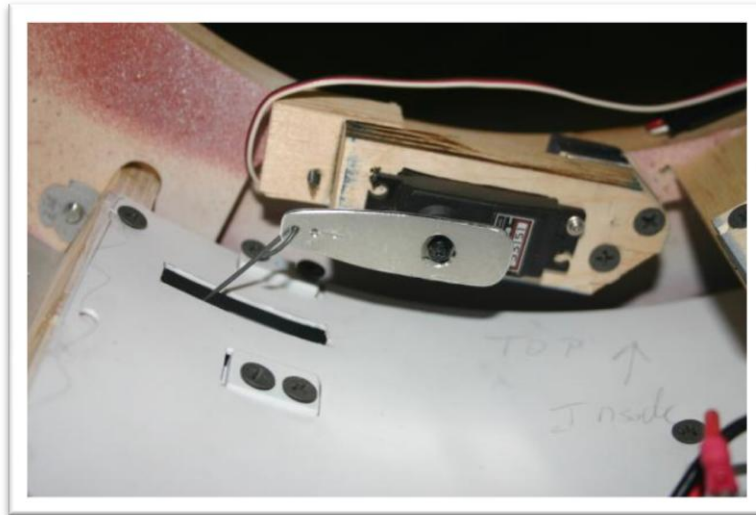
Figure 36: Utility arms mechanized with a servo
