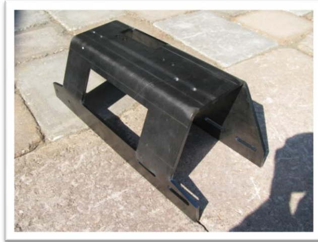
Figure 42: R2-X2 eXperimental steel foot drive shell - Photo by: Blake Mann
