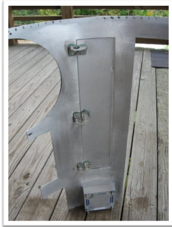
Figure 38: Back door (inside view) hinged with Robart hinges - Photo by: Chip Luck
