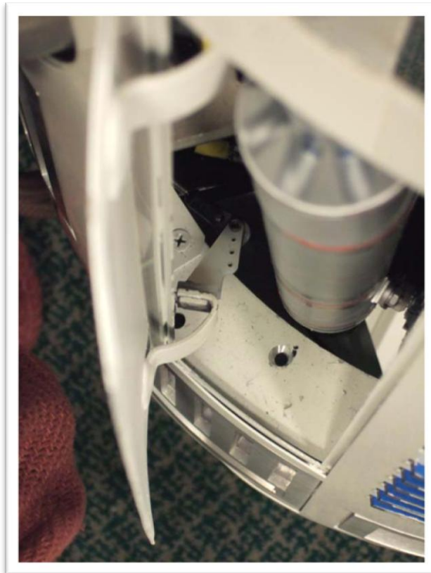
Figure 41: Front door panel mechanized with a servo
