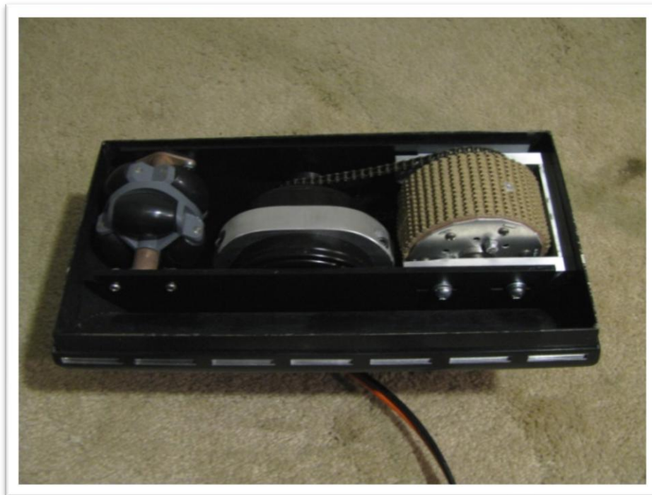
Figure 48: R2-X2 eXperimental foot drive assembled - Photo by: Blake Mann
