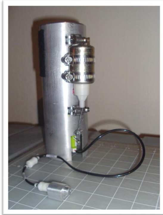
Figure 5: Compressed air can upside down with solenoid trigger - Photo by: Tiny P.
