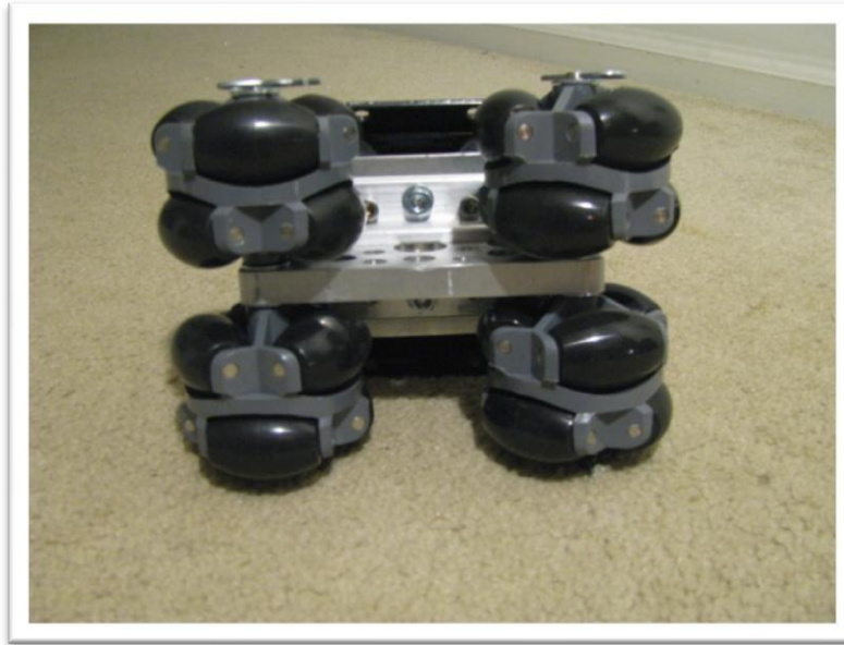
Figure 57: Stabilizer foot omni wheel platform - Photo by: Blake Mann
