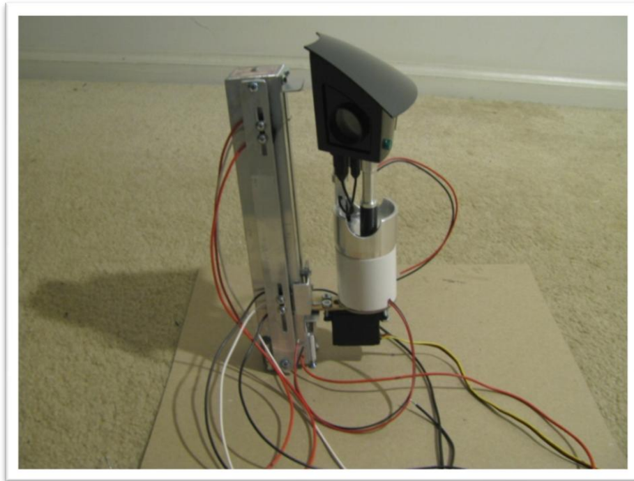
Figure 20: Custom periscope lifter – periscope mounted on servo base socket
