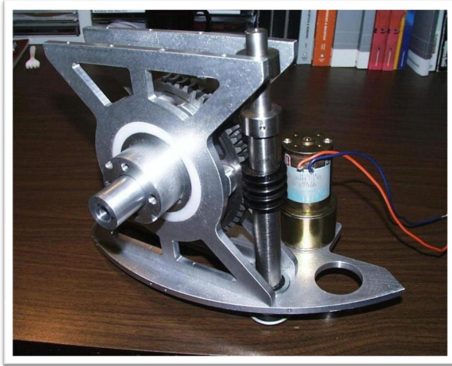
Figure 71: Shoulder rotation worm gear - Photo by: Dave Painter
