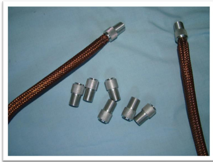
Figure 66: Battery cable protective hoses
