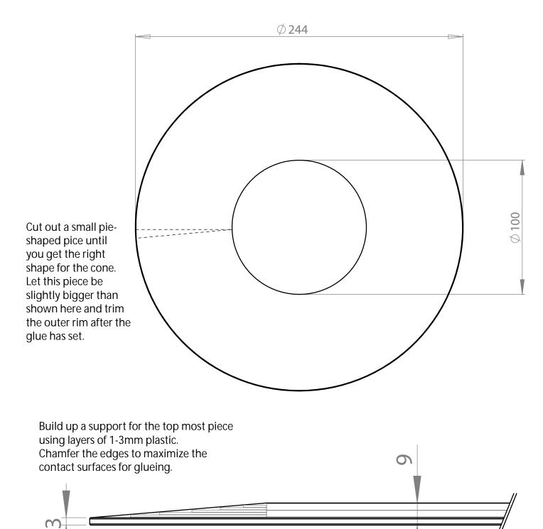
As an alternate to this method would be using filler instead of the "pie" cut top shape and then carefully sand down to correct shape. I have not tried this, but it should work.
