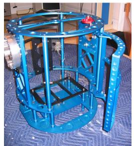
Figure 4: COM-8 Frame before adding the 2-3-2 mechanism.
