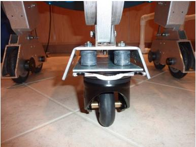
Figure 23: Rubber mounts are inserted between the caster place and the foot shell for shock absorption.
