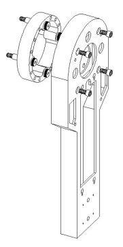
Figure 9: Modified leg to flange assembly.
