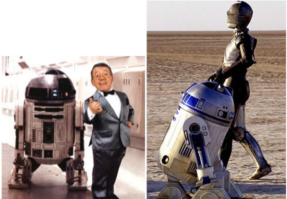
Figure 1: Left: Kenny Baker and his R2-D2 in 2-leg configuration. Note the tube extensions connecting the underside of the body to the foot shells for the actor's feet. Right: R2-D2 rolling around in his familiar 3-leg configuration.
