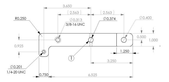
Figure 8: J-bar dimensions. This J-bar is intended for a 3" stroke actuator. The bar is 0.375" thick.
