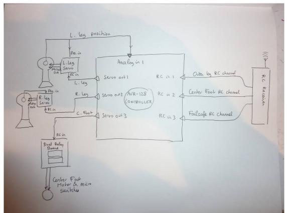
Figure 24: 2-3-2 control architecture
