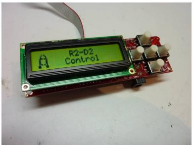
Figure 25: Olimex AVR-MT-128 microcontoller board
