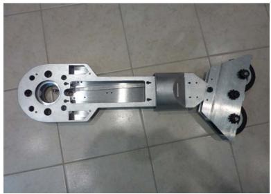
Figure 11: Outer leg. Note the narrow steel bar running from the foot to the shoulder opening and used for foot angle locking.
