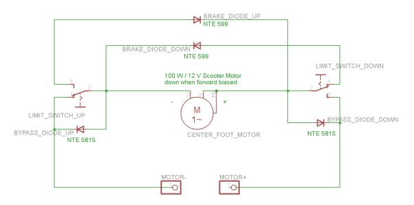
Figure 21: Limit switches and diodes for the end travel control. The two large NTE599 15A cont / 250A max diodes are for braking at travel end.
