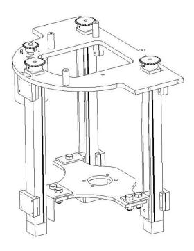
Figure 15: Center leg lift mechanism
