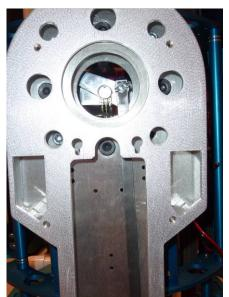
Figure 13: The top of the ankle tie rod is attached to a pin near the shoulder center of rotation.
