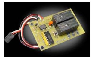
Figure 20: RCE220 RC Small Dual Relay Switch from robotmarketplace.com
