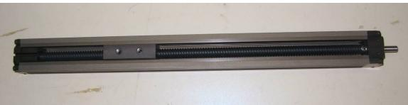
Figure 16: PCB Linear MLD actuator, part number MLD028D-0AJ201-0338-000. It has a 338mm main body length and a 10 mm lead screw.
