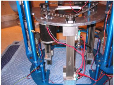
Figure 18: View of the leg lift mechanism during assembly.
