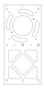
Figure 5: Shoulder mounting plate that comes with the COM-8 frame, showing the 4 curved 48° openings.
