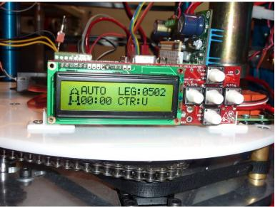
Figure 28: Controller display in auto mode. The outer legs have been commanded in 2-leg position, as indicated by the close to 500  $\mu$ s leg channel value read from the RC transmitter. Accordingly, the center leg has been brought to up (U) position. A cumulative run-time counter is at the lower left – R2 has been up for less than a minute and still shows 00:00.
