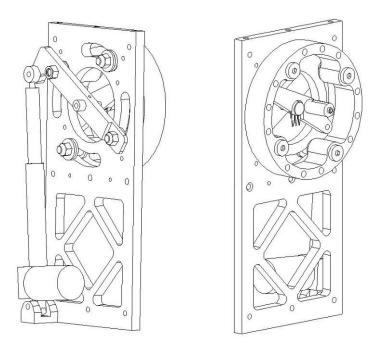
Figure 3: Views of CuriousMarc's R2-D2 shoulder actuation mechanism
