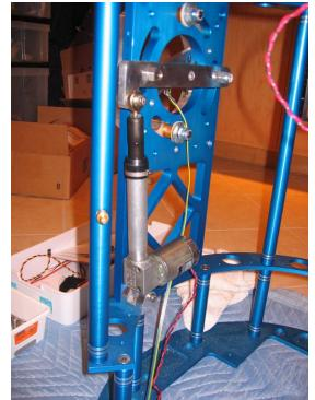
Figure 7: Actuator installed in the frame, connected to an anchor at the bottom and to a J-bar at the top.
