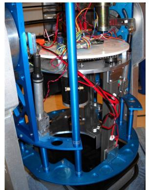
Figure 19: Completed Leg Lift mechanism.
