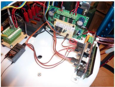
Figure 27: Close-up view of the electronics. RC receiver to the left, outer leg servo controller to the top, microcontroller to the right.
