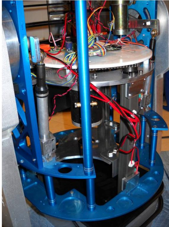
Figure 19: Completed Leg Lift mechanism.
