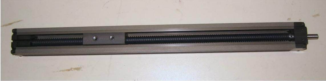
Figure 16: PCB Linear MLD actuator, part number MLD028D-0AJ201-0338-000. It has a 338mm main body length and a 10 mm lead screw.
