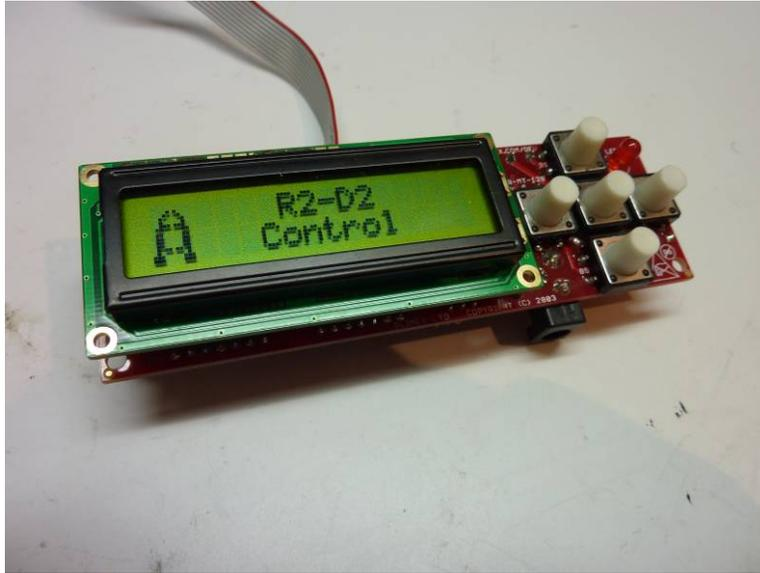
Figure 25: Olimex AVR-MT-128 microcontroller board
