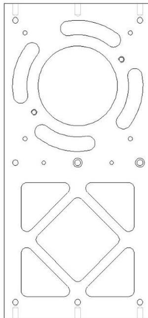
Figure 5: Shoulder mounting plate that comes with the COM-8 frame, showing the 4 curved 48° openings.
