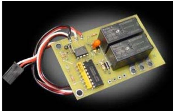
Figure 20: RCE220 RC Small Dual Relay Switch from [robotmarketplace.com](http://robotmarketplace.com)
