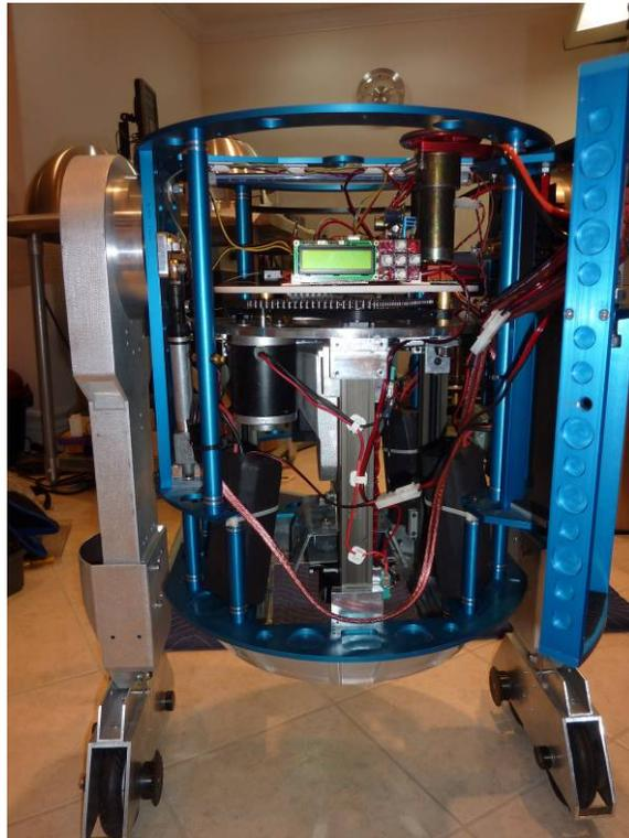
Figure 30: Finished 2-3-2 installation. Note the batteries in temporary position for balance trials. Eventually I settled on two batteries in the back door and one in the front.
