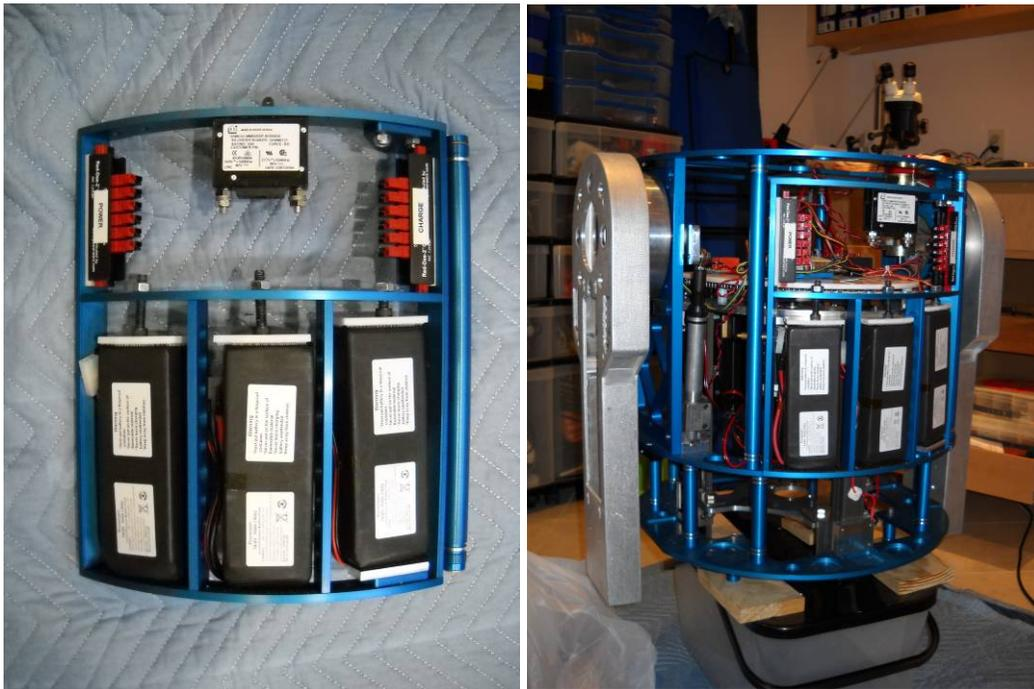
Figure 29: 3x 14.8V/10Ah Lithium Polymer batteries fit in the back door.
