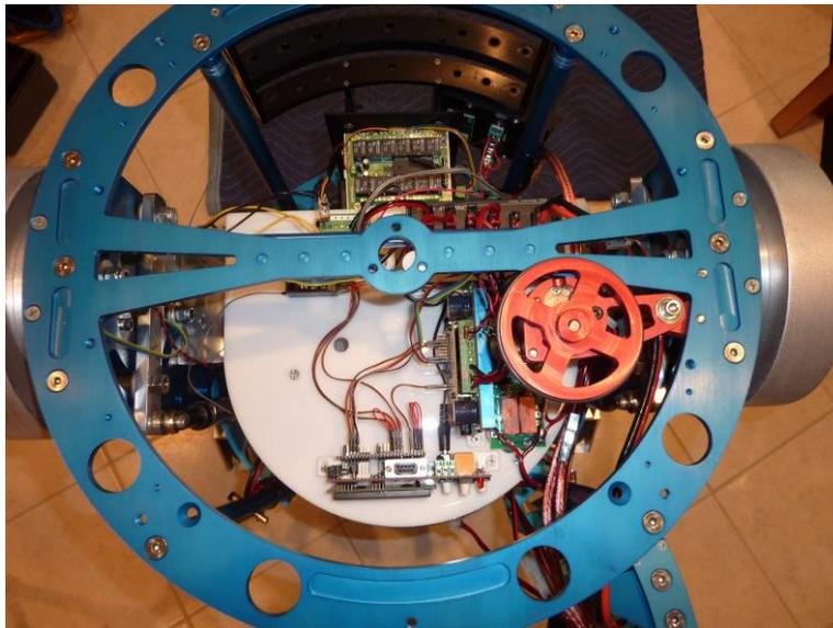
Figure 26: View of the installed electronics. Controller is at the bottom, to the right is the outer leg servo controller. The relay board for the center foot is partially visible under the dome wheel.
