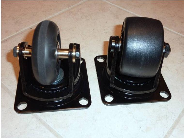
Figure 22: Misumi casters, with the original hard wheel at right, and grafted with a soft neoprene wheel at left
