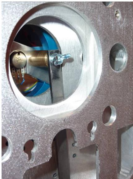
Figure 14: Detail of the top attachment pin for the tie rod.
