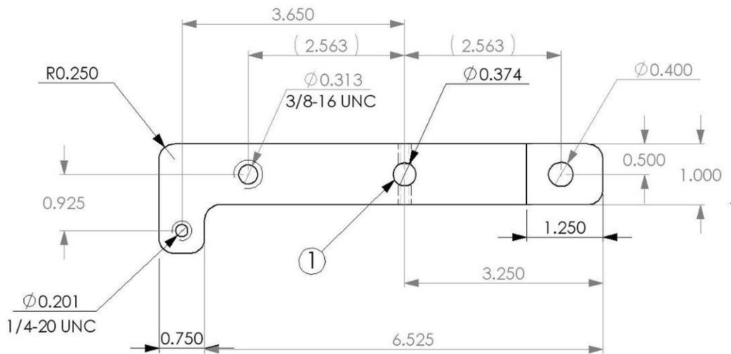
Figure 8: J-bar dimensions. This J-bar is intended for a 3" stroke actuator. The bar is 0.375" thick.
