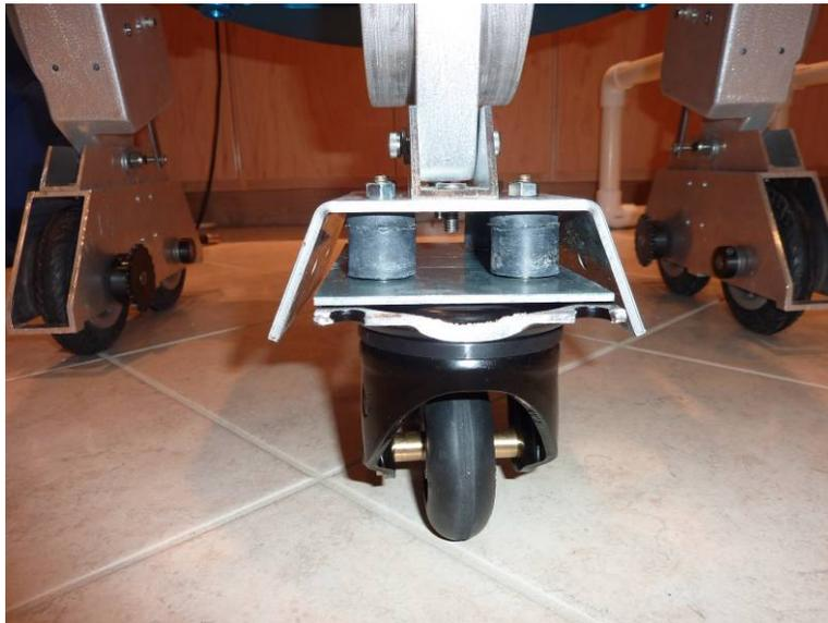
Figure 23: Rubber mounts are inserted between the caster plate and the foot shell for shock absorption.
