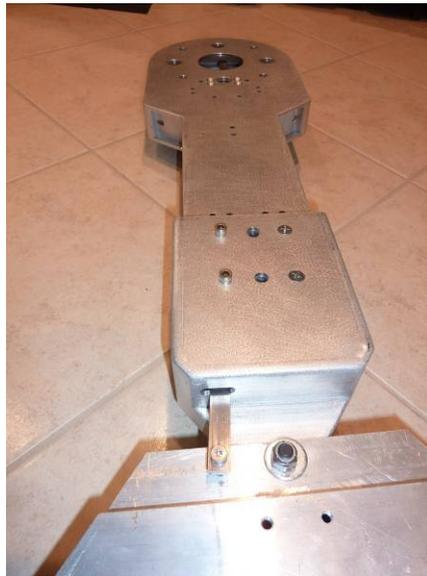
Figure 12: Lower portion of the outer leg. The ankle tie rod goes through a small opening at the bottom of the ankle and is attached to an anchor screw on the foot shell.
