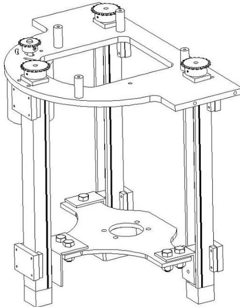
Figure 15: Center leg lift mechanism
