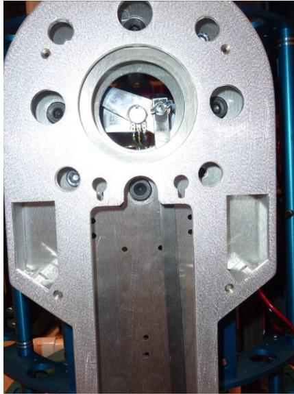
Figure 13: The top of the ankle tie rod is attached to a pin near the shoulder center of rotation.
