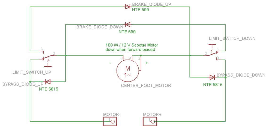
Figure 21: Limit switches and diodes for the end travel control. The two large NTE599 15A cont / 250A max diodes are for braking at travel end.
