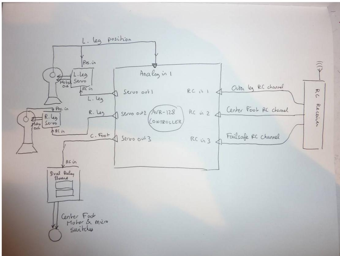
Figure 24: 2-3-2 control architecture
