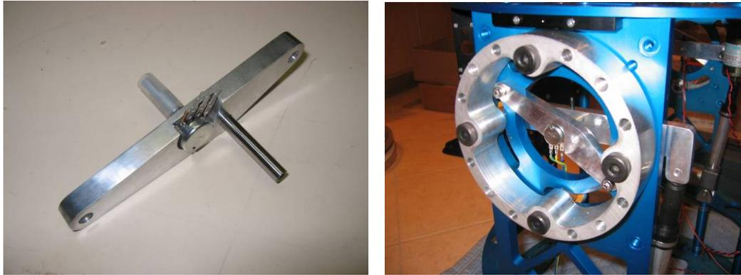
Figure 10: Spanner with the potentiometer and anchor pin attached (left), spanner mounted on the outside of the shoulder plate (right).
