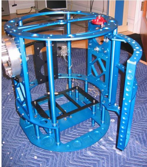
Figure 4: COM-8 Frame before adding the 2-3-2 mechanism.
