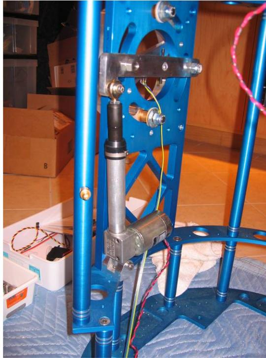
Figure 7: Actuator installed in the frame, connected to an anchor at the bottom and to a J-bar at the top.
