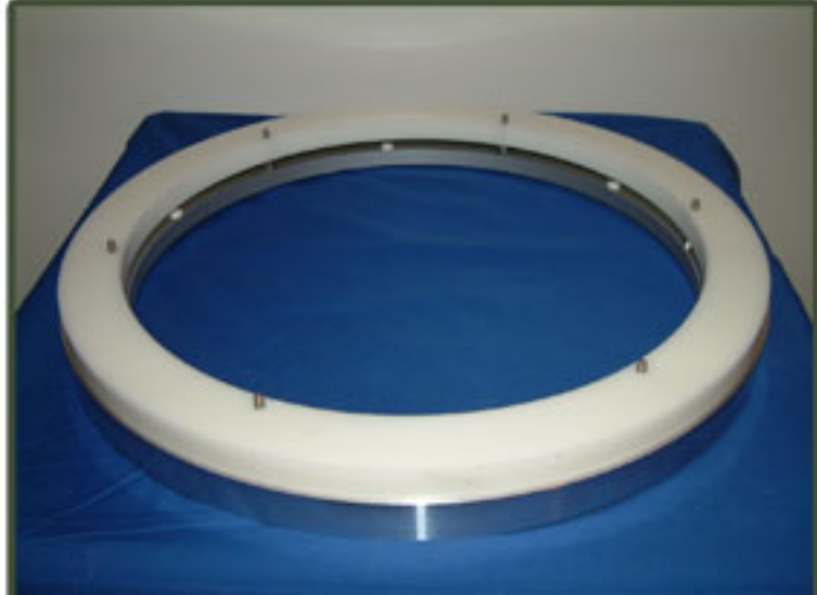
The Rockler bearing connected to the aluminum ring with plastic ring on top
