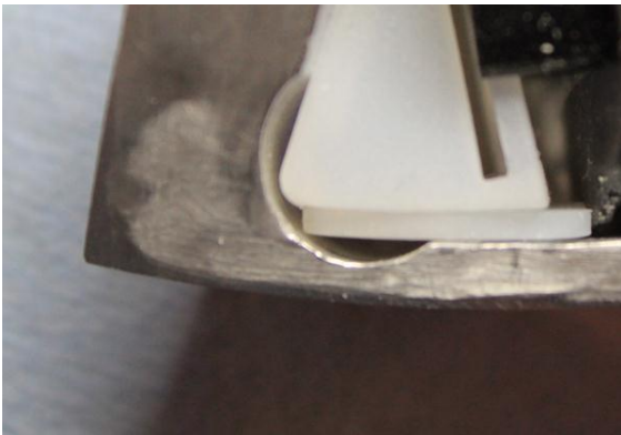
Rubber Spacer between Wedge and Housing
